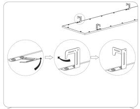
4.Rotate the clips, unbend the bracket, make it perpendicular to the lamp. Rotate the bracket by 90 degrees.
