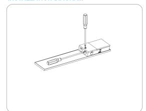
Open the driver junction box and knock off the quantity of knockouts needed.
