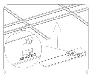
2. Switch the color temperature and power selector to the required setting and then push it into T box.
