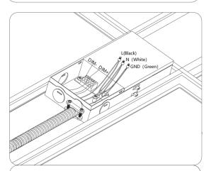
Connect the cable to the driver junction box as per labeling wire diagram. Connection Instruction: For dimming wires use the correct tools to press the terminal and pull the wires into the terminal and then release, connect AC wires and ground wires with rated wire nuts.
